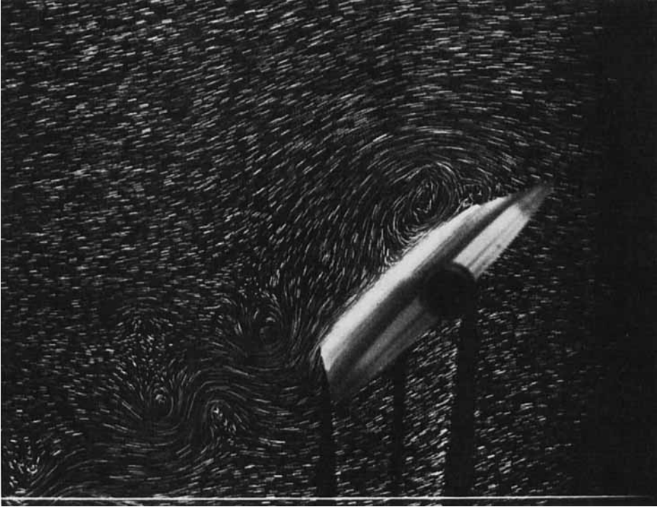
FIGURE 3. Visualization of a rapidly oscillating elliptic airfoil in an impulsively generated parallel flow; Re = 3000 , f^* = 1.0 , \bar{\alpha} = 30^\circ , \Delta\alpha = 15^\circ , \alpha_0 = 15^\circ , t^* = 1.25 .
